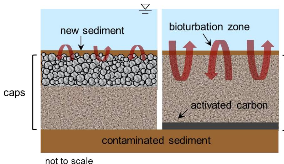
When designing and constructing conventional or active isolation caps, additional site- and sediment-specific factors should be considered, including: potential influence of groundwater upwelling, geotechnical stability (sediment bearing strength and slope stability), and gas ebullition. Possible use of geotextiles in cap design should also be carefully considered.
