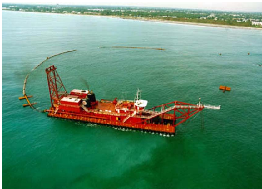
Figur 4-2. Sugmudderverk med rörledningssystem, Palm Beach Nourishment Project, Florida. (www.pbcgov.com/erm/divisions/enhancement/beach1.htm) dec. 2004.
