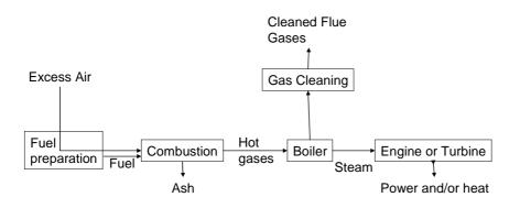
Figure 6. Flow chart of a conventional combustion system (based on Figure 2 in (Schuck, 2006)).
