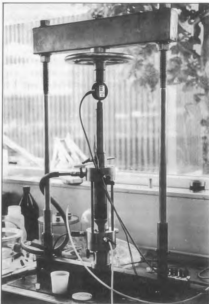
Calibration chamber with probe mounted in the loading frame
