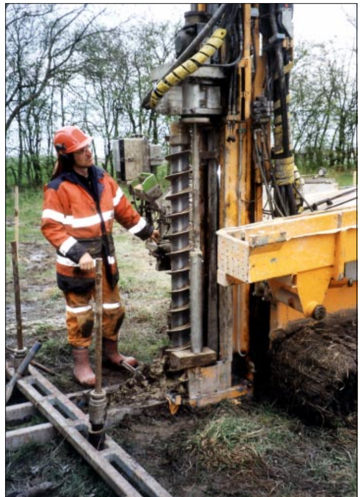
Fig. 50. Sampling operation with tube sampler in progress. The hollow stem auger is rotated down and the prepared tube sampler is suspended at the side, ready to be lowered into the shaft.
