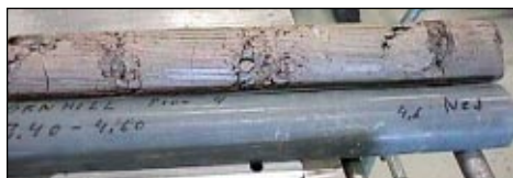
c) core from 3.9 to 4.6 metres depth showing clay till mixed with layers of gravelly soil
