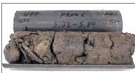
d) core from 5.3 to 5.8 metres depth showing gravel and cobbles in the mixed till layer
