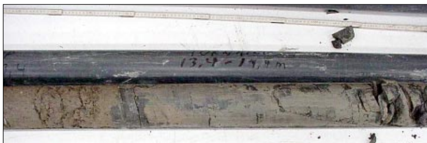
h) core from 13.6 to 14.8 metres depth showing the transition from North-east clay till to bedrock of clay shale
