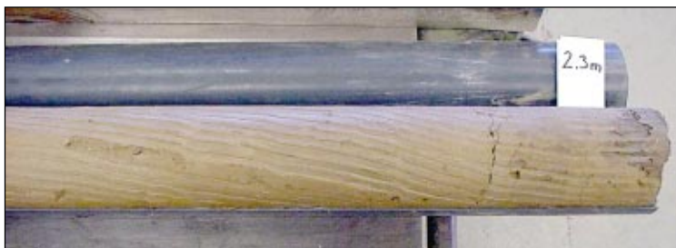
b) core from 1.7 to 2.3 metres depth showing homogeneous clay till
