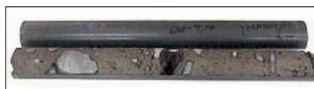
f) core from 6.5 to 7.5 metres depth showing gravelly, silty clay till with cobble size particles at the top of the North-east till
