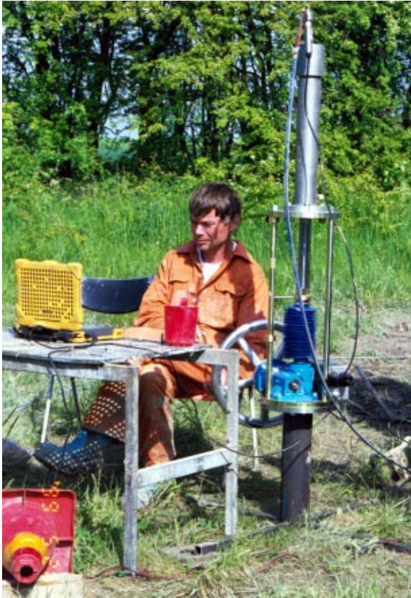
Fig. 29. Performing a test with the new pressuremeter at Tornhill.
