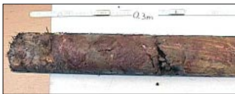
a) core from 0 to 0.5 metre depth showing the transition from top soil to Baltic clay till
