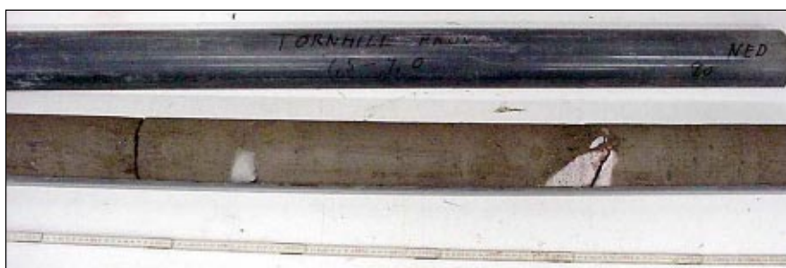
g) core from 7.5 to 9.0 metres depth showing sandy, silty North-east clay till with infusions of cobbles
