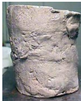
Fig. 73. The specimen from 3.8 metres depth after testing.
