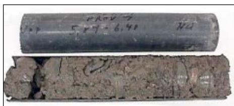
e) core from 5.9 to 6.5 metres depth showing sandy, gravelly till at the bottom of the layer of mixed till
