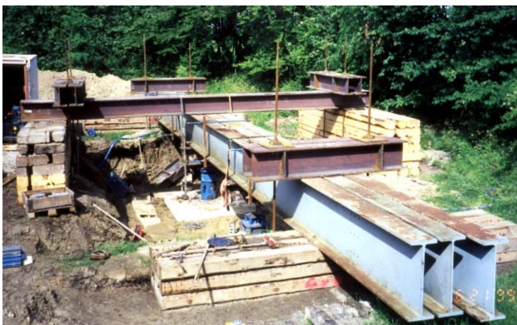
Fig. 82. Reaction system being mounted.
