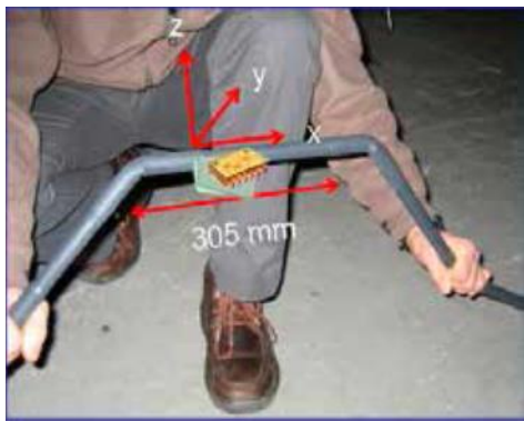
Figur 3.8 SAAF (ShapeAccelArrayField). Versatile rope-like array of sensors for Geotechnical applications. (Från Cautus Geo AS 2013).
