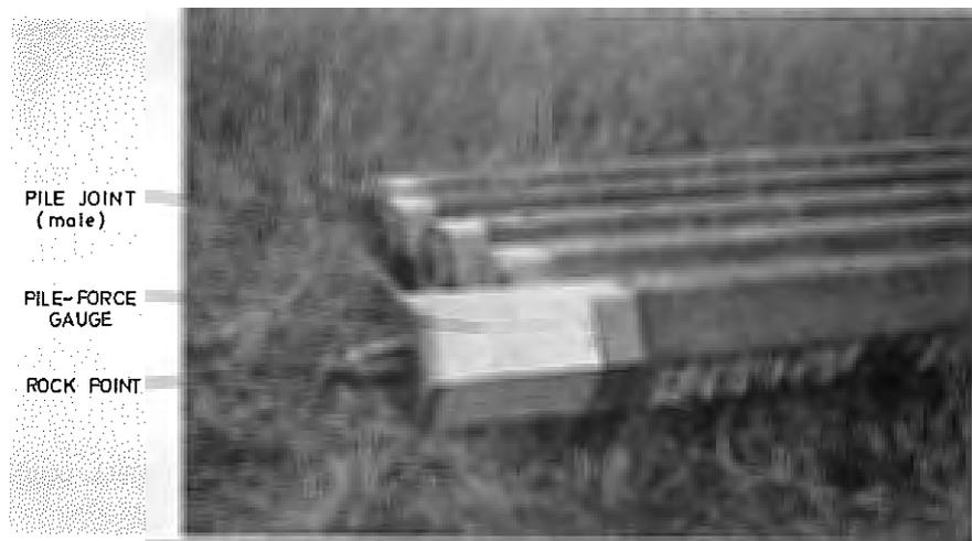
FIG. 3. Pile-force gauge mounted on a pile tip and equipped with a rock point.
