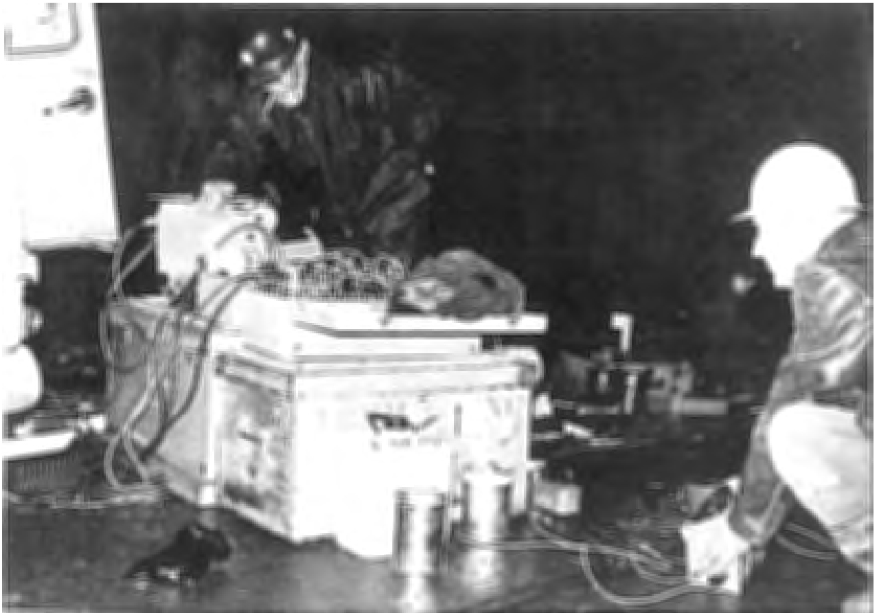
Fig. 3 Detonating and recording equipment for tunnel seismic refraction measurements.
