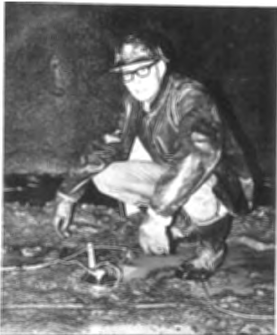
Fig. 2 Geophone-steel plate pickup for tunnel measurements. Hall-Sears seismometer, spring suspension, moving coil type, frequency response range 5-300 cps; pickup spacing 1-5 m.
