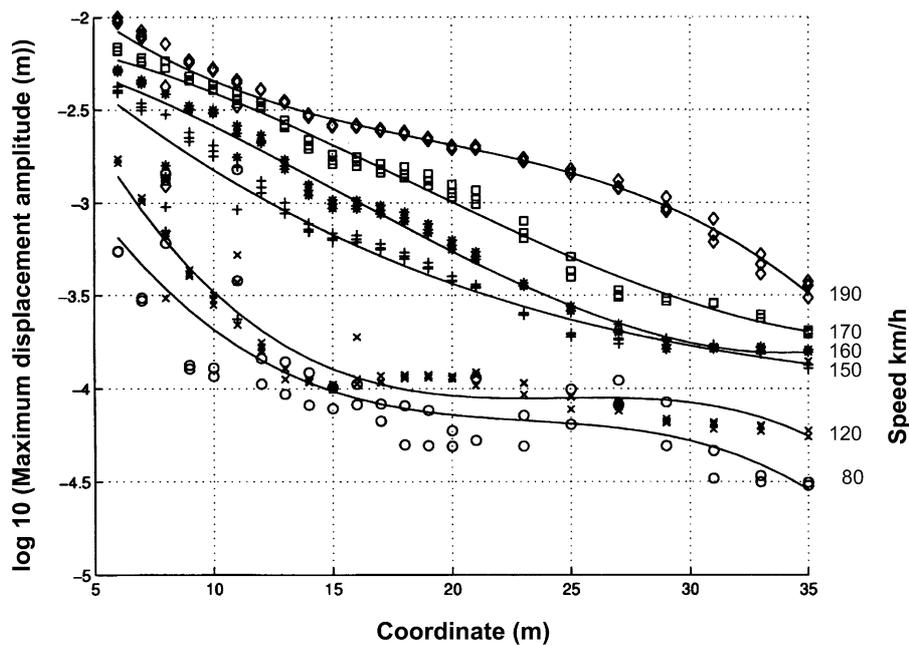
Fig. 28. Maximum displacement amplitudes with distance from track and train speed before countermeasures, CTH (2001).
