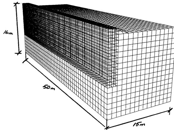
**Fig. 10. FLAC3D model used in the analyses of dry DMM improvement.**
