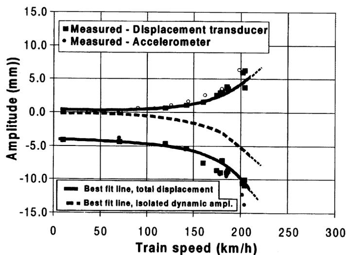
Fig. 2. Downward displacement of the track at different train speeds (lower solid line), lift (upper solid line) and dynamic (vertical) contribution (dashed line) at Ledsgård. Banverket (1999)
