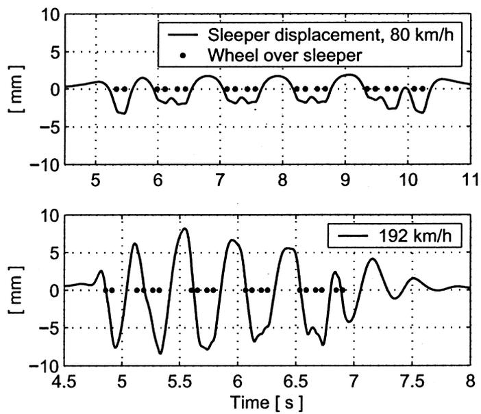
Fig. 25. Displacement of one sleeper end during train passage at speeds of 80 and 192 km/h.
