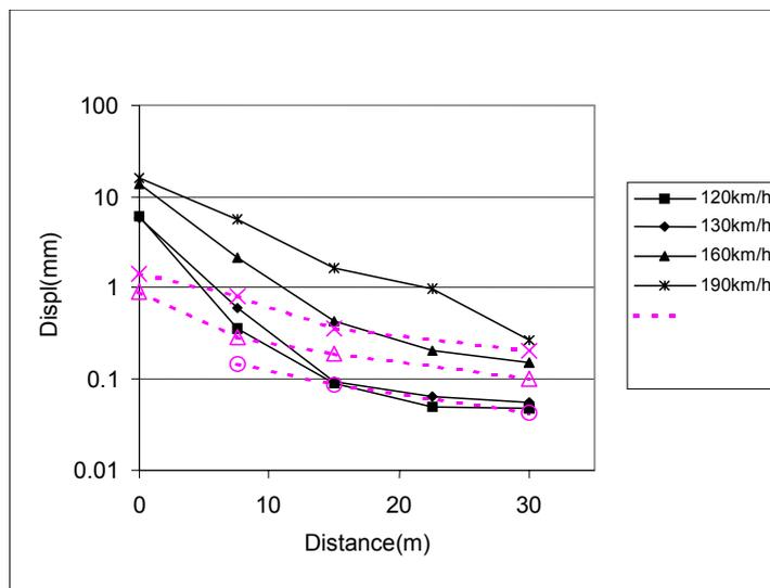
**Fig. 27. Attenuation of particle displacement (peak-to-peak) with distance from the mid-point of the western track at different train speeds before (solid lines) and after (dashed lines) dry DMM soil improvement, KTH (2001).**
