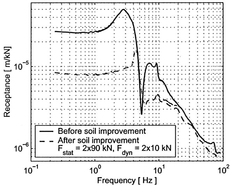
Fig. 24. Track receptance of the western track before and after dry DMM improvement.
