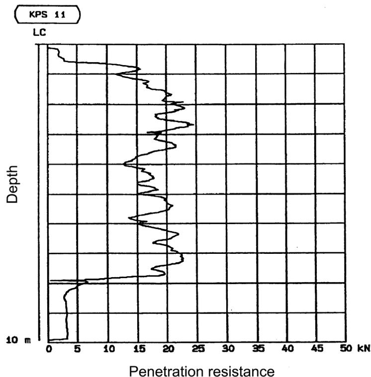
**Fig. 18. Result of field test on a dry DMM column. Penetration resistance of pre-bored standard column penetration test (SCPT).**
