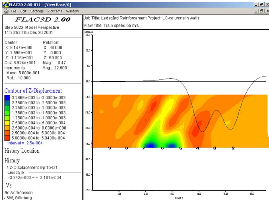
**Fig. 11. Results of FLAC3D analyses of a two-bogie load travelling along the symmetry line at 55 m/s - unreinforced track above and dry DMM improved below. Deflection pattern on the surface shown together with deflection history at registration point 4.**
