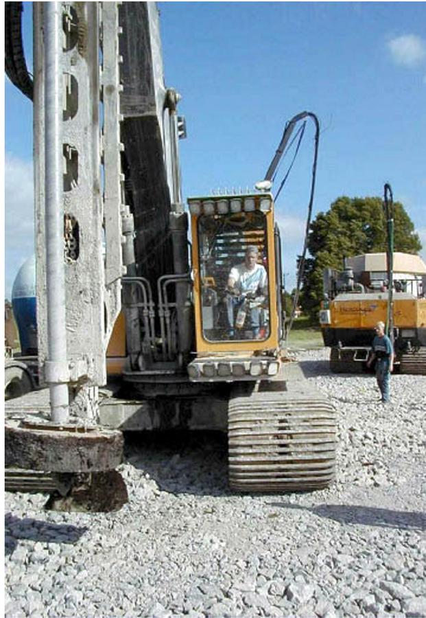
**Fig. 15. Limix rig for soil improvement with the dry deep mix method.**
