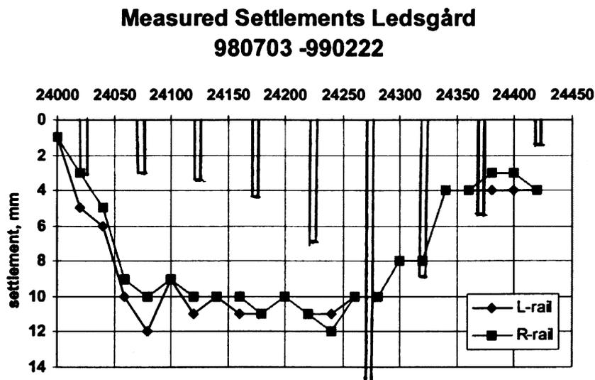
Fig. 7. Settlement observations of the western track at Ledsgård (both rails) together with relative vibration levels along the studied section.
