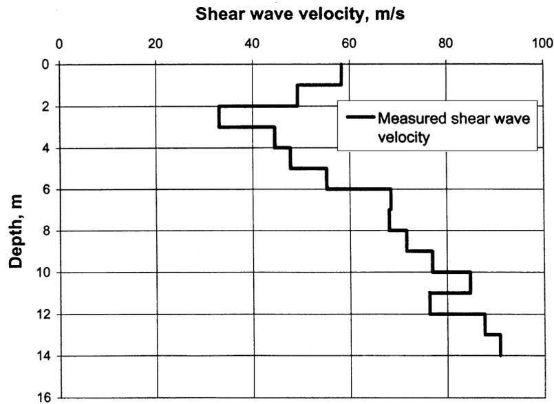
Fig. 5. Shear wave velocity at Ledsgård.
