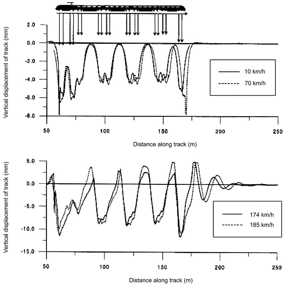
**Fig. 22. Measured vertical displacement at different speeds at Ledsgård.**
