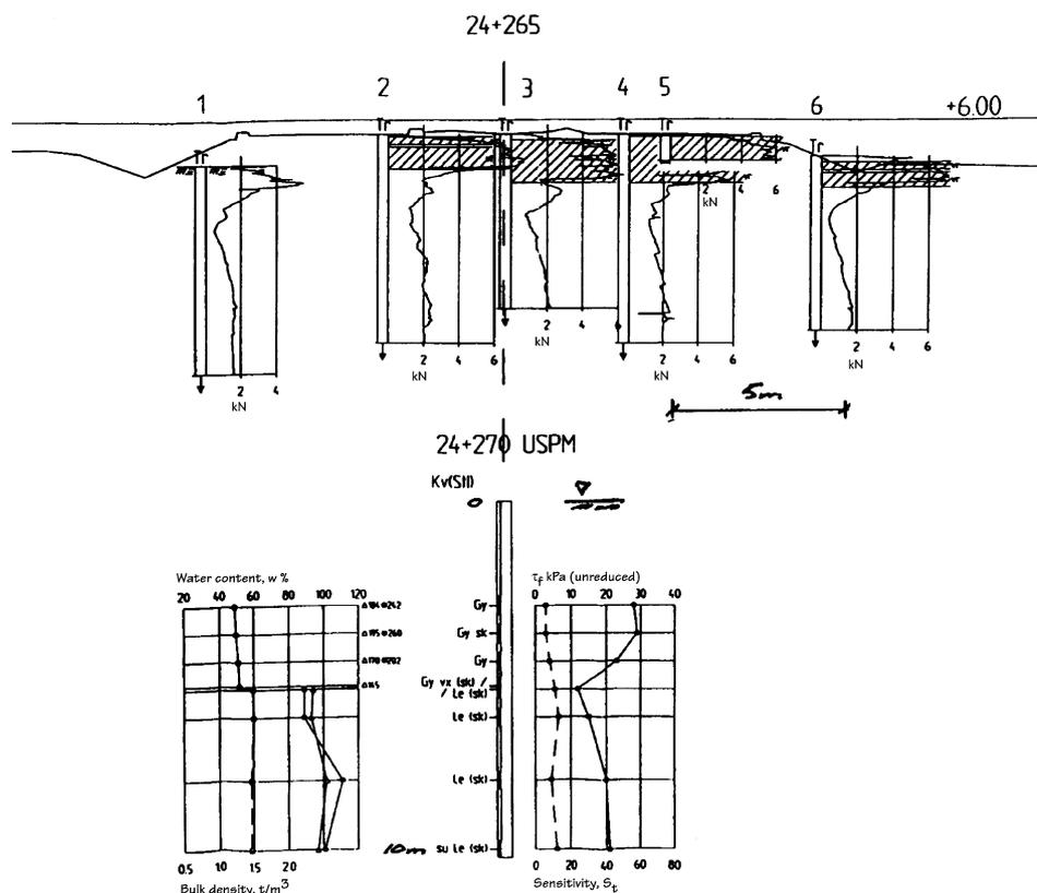
Fig. 4. Soil conditions in the Ledsgård test section.
