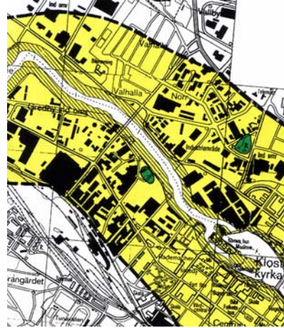
Figure 4.1a "The Manuel" Map, Stage 1a, performed according to the in Sweden commonly used method for manually performed overview landslide mapping. Extract from the manual overview mapping carried out in Eskilstuna, SRSA /Bohusgeo [1996]. Legend, see below.
